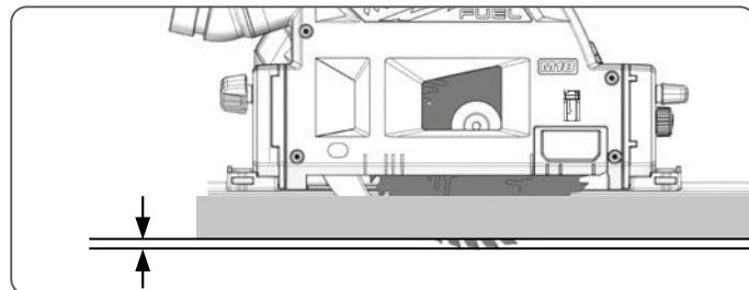
Adjust the cutting depth to the thickness of the workpiece. Less than a full tooth of the blade teeth should be visible below the workpiece.
